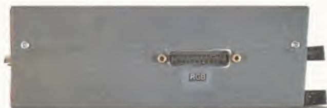
If you're tired of the blurry composite or RF TV output from your CD 32 then the SX-1's RGB connector will be a real bonus.
